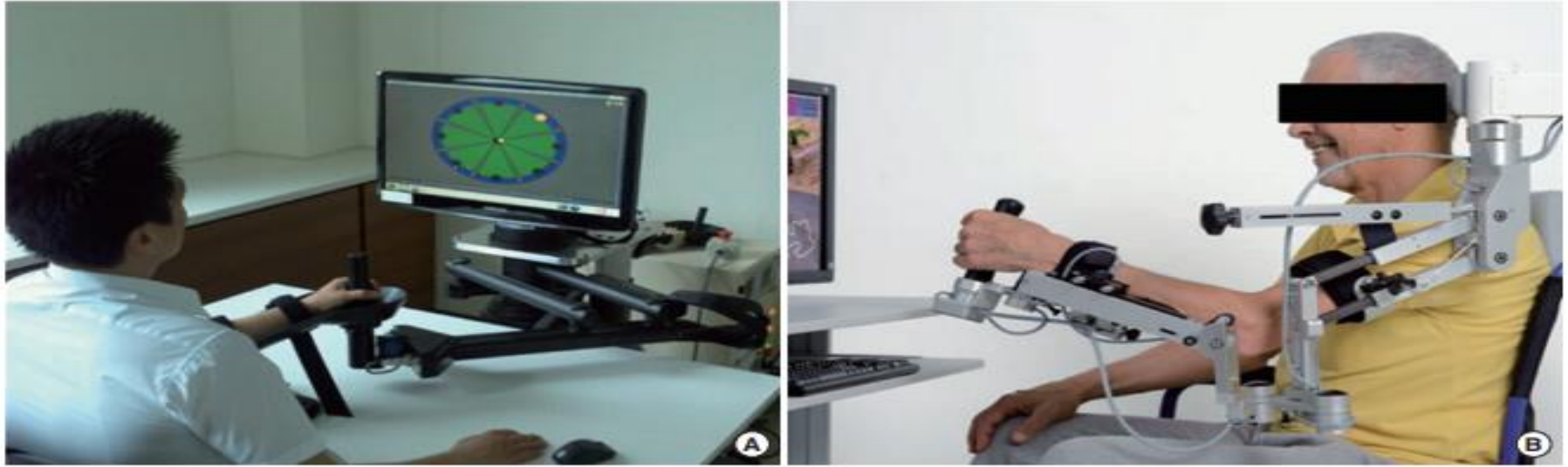
Figure 1. Examples of robotic devices for motor training (A) End-effector type (InMotion 2.0 Interactive Motion Technologies, Watertown, MA, USA), (B) Exoskeleton type (Armeo®, Hocoma, Switzerland).
